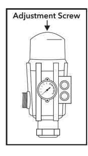
To change the pump start pressure (cut-in) adjust The screw on the top of the controller
